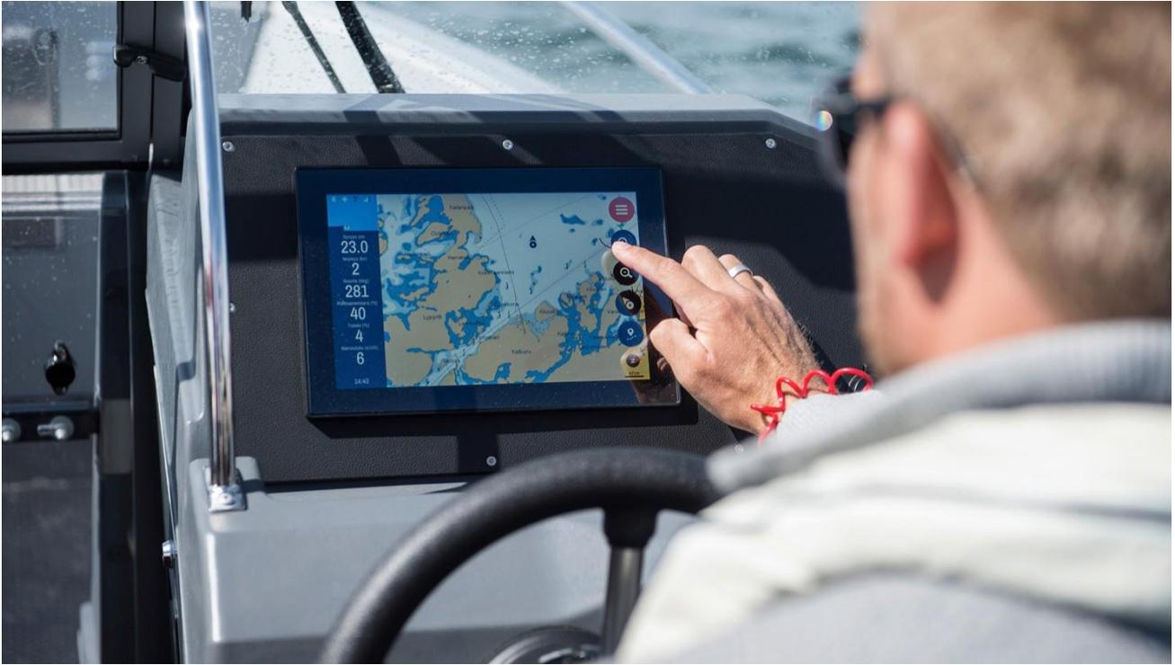
The large touch screen incorporates electronic charts, an on-board computer and an entertainment system into the motorboat as part of the standard equipment.
